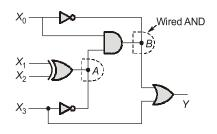
Out of 16 possible combinations of  $X_3 X_2 X_1 X_0$ ,  $X_3$  will be high for 8 combinations. So, Y will be high for 8 combinations.
