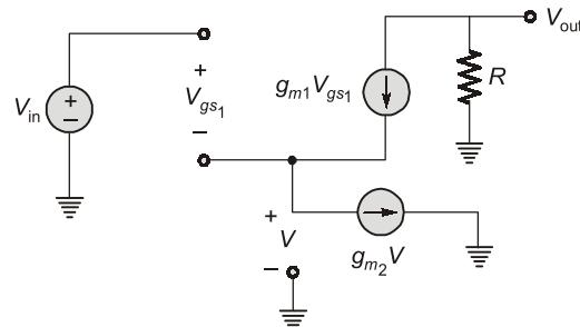
$$\begin{aligned} \text{Substituting } V &= -V_{gs2} \\ \text{now, } V_{in} &= V_{gs1} + V & \dots(i) \\ \text{and } g_m1 V_{gs1} &= g_m2 \cdot V & \dots(ii) \\ (\because \text{from KCL at node } S_1) \end{aligned}$$
