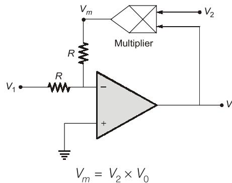
$$V_m = V_2 \times V_0$$
