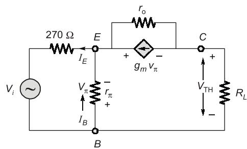
$$V_\pi = -V_i \times \frac{r_\pi}{r_\pi + 270}$$
