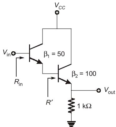
$$R' = r_\pi + (\beta_2 + 1)R_E \\ = 1\text{k} + (101)(1\text{k}) = 102\text{ k}\Omega$$
