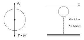
$F_{\text{buoyancy}} = \text{Tension} + \text{Weight}$
