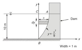
Horizontal force  $(F_H)$ :  $F_H = \rho g \, \overline{h} \, A_v (\rightarrow)$   $= \left(10^3\right) \left(9.81\right) \left(\frac{10}{2}\right) (10 \times 1)$   $= 490.5 \, \text{kN} (\rightarrow)$   $F_V = \rho g \forall$   $= (10^3) (9.81) \times (\text{Area of ABC}) \times \text{Width of dam}$   $= \left(10^3\right) \left(9.81\right) \left[\int_0^{10} x \, dy\right] \times 1$   $= \left(10^3\right) \left(9.81\right) \left[\int_0^{10} \sqrt{9y} \, dy\right] \times 1$
