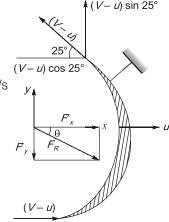
Force exerted by the jet in the direction perpendicular to direction of jet, per unit weight
