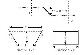
$$F_1 = \frac{V_1}{\sqrt{gA/T}} = \frac{2.182}{\sqrt{\frac{9.81 \times 27.5}{6 + 2 \times 2 \times 2.5}}} = 0.531 < 1$$
