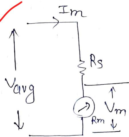
$$\therefore R_s \text{ (multiplier resistance)} = R_m (m-1) = 100 (36-1) = 3.5 \text{ k}\Omega$$
