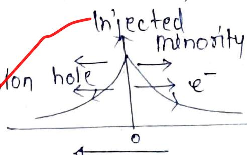
$$\frac{d}{dx} J_n(x) \Big|_{x=0} = 0 + \left( \frac{-\Delta P}{L_p} \right) = -\frac{n_i^2}{L_p \times N_D} e^{V_D/V_T}$$
