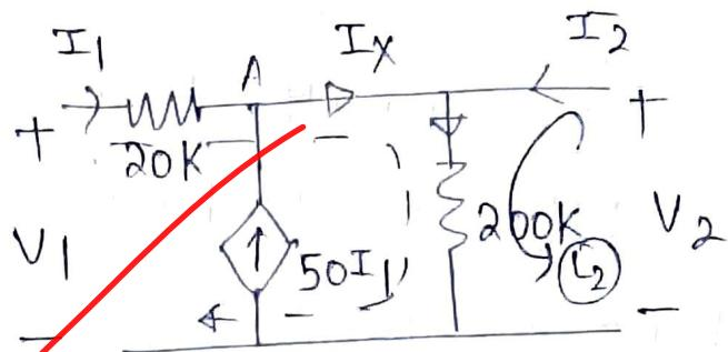
$$\boxed{\begin{aligned}V_1 &= h_{11}I_1 + h_{12}V_2 \\I_2 &= h_{21}I_1 + h_{22}V_2\end{aligned}}$$
