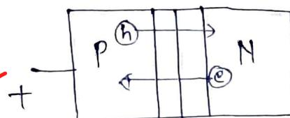
where,  $I_{PE}$  denotes hole current crossing the JE from P to N side, which is diffusion current.
