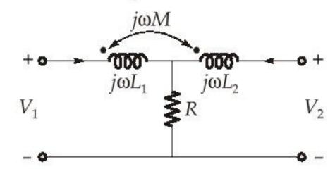
(ii) For the circuit shown, what should be the value of load resistor  $R_{Load}$  so that it absorbs maximum power and then, what would be the power absorbed by  $R_{Load}$ ?
