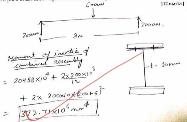
Shear flow =  $\frac{VAy}{I}$   $V = \frac{600}{2} = 300 \text{ mV}$ , 9 = 300×103 200×10]× 205 330.01N/mm 372.71×106 Thus, for a fitch of 200 mm, assuming 2. vivet in each fitch length, force on 2 rivets = 330.01×200 = 66 km Thus design force on each rivet 6 = 33 WN.
