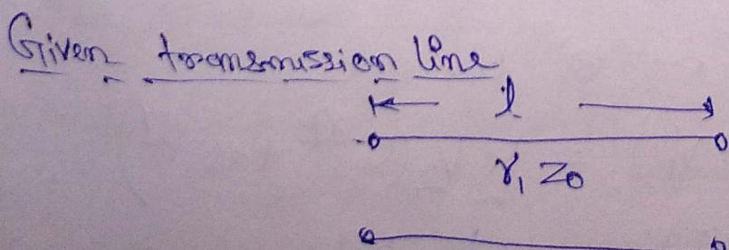
To find  $A = \frac{V_1}{V_2} \Big|_{I_2=0}$  and  $C = \frac{I_1}{V_2} \Big|_{I_2=0}$
