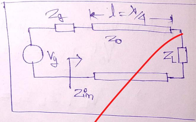
Input impedance of the given line (lossless).
