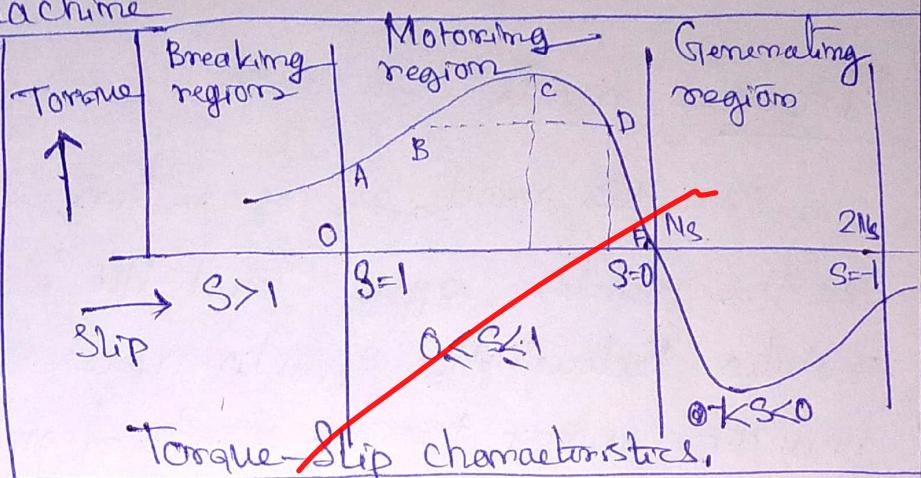
The torque Slip - characteristics of 3-Φ induction machine shown above, in which for  $s > 1$  induction machine works as in breaking mode, and for  $0 \leq s \leq 1$  works as motor and for  $-1 \leq s \leq 0$  works as generator.
