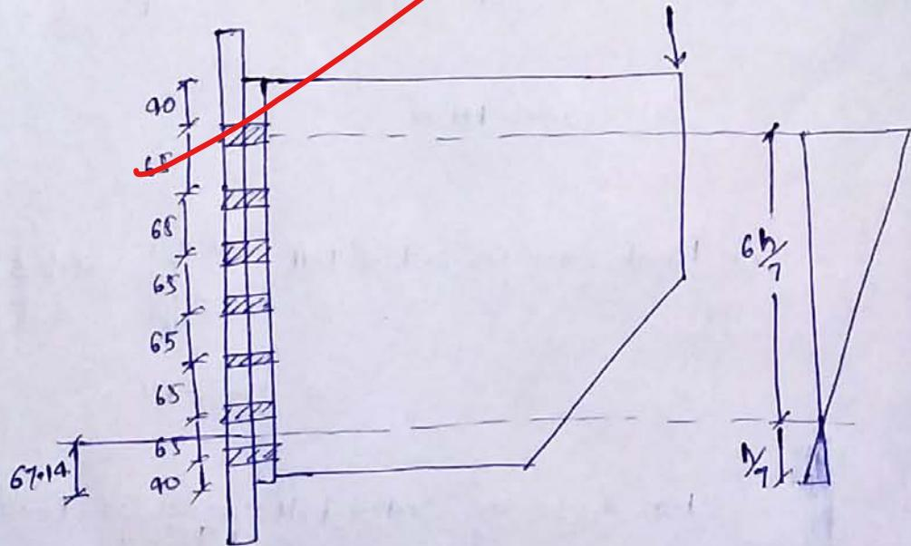
$$\text{Total depth of bracket} = h = 65 \times 6 + 2 \times 40 = 470 \text{ mm}$$
