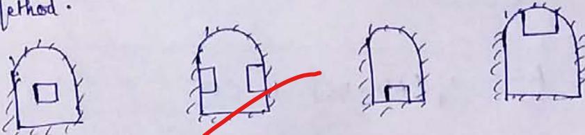
The tunnelling is carried out by driving the drift portion first. It may be classified as top drift, bottom drift, central drift depending on the relative position with respect to main bore. First the small section is driven and further widened. It is used as a correction measure for water table. Also, timber installation of support become easy. The drift is used as a ventilation. But it is costly and main bore can't driven until the drift portion is completed.
