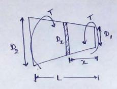
Assuming on element of diameter Dx at a distance of x from smaller dia end.
