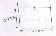
Area  $A_1 = B \times Y_1 = 2 \times 7.5 = 15 \text{ m}^2$ Perimeter  $P_1 = 7.5 + 2 \times 2 = 11.5 \text{ m}$ .\*. hydraulic Padius  $P_1 = \frac{A_1}{P_1}$  $= \frac{15}{11.5} = 1.304 \text{ m}$
