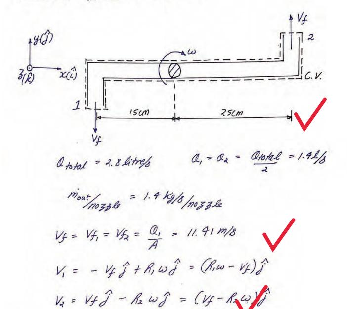
Extension resisting torque  $T_R = 0$ (i) Zero resisting torque  $T_R = 0$   $EM_0 = 0 \hat{k} = L_{out} - V_{in}^{0}$  (consentation of angular momentum)
