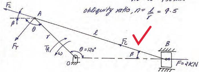
In DOAB, by sine rule => sing = sing > B= 11.09° force transmitted to connecting rod, Fe = F => Fc = 2.038 KN from the diagram, crank effort, FT = Fc sin (0+18) => FT = 1.536KN ... The resisting torque on crank TR = TFT ⇒ TR = 153.6 N-m (CW) .. The resisting torque required at the crank in order to keef the mechanism in Static equilibrium is 153. 6N-m in Clockwise direction.
