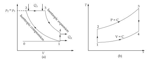
Here, the volume ratio  $\frac{V_1}{V_2}$  is the compression ratio, *r*. The volume ratio  $\frac{V_3}{V_2}$  is called the
