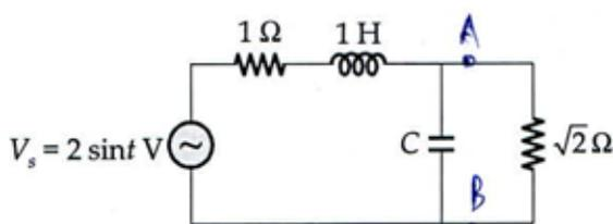
Load is fixed and source impedance is variable. Now  ~~$X_{Th}$  across  $\sqrt{2} \Omega$  should be minimum~~ so across A & B finding  $V_{Th}$  &  $R_{Th}$ . [10 marks]
