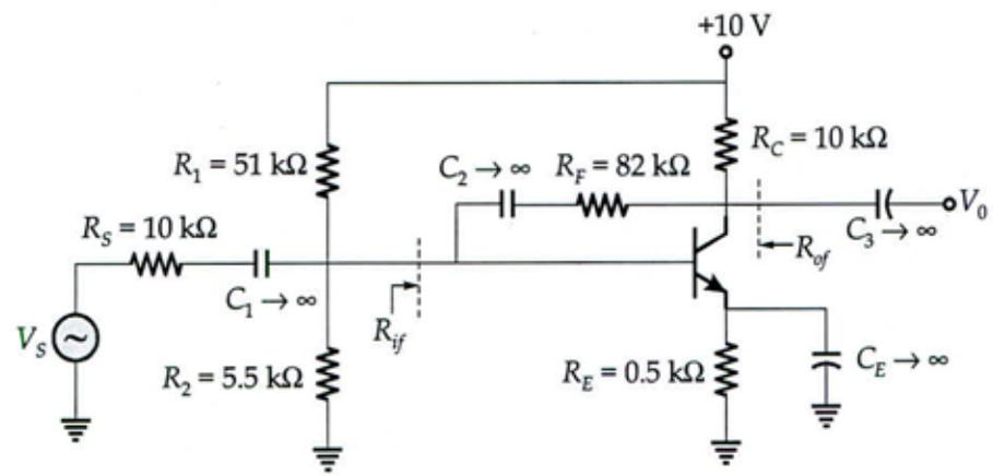
If  $\beta = 100$ ,  $V_{BE(on)} = 0.7\text{ V}$  and  $V_A = \infty$ , then calculate the small signal input resistance  $R_{if}$  and small signal output resistance  $R_{of}$  (Assume  $V_T = 26\text{ mV}$ )
