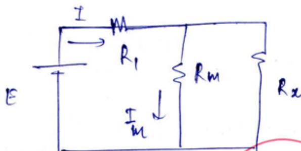
$$I_m = \frac{R_x}{R_m + R_x} \times \frac{E(R_m + R_x)}{R_m(R_1 + R_x) + R_1 R_x}$$
