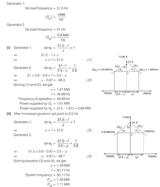
(iii) For the load transfer from generator '1' to generator '2' without changing system frequency, generator '1' must be operating at no load at frequency f = 50.11 Hz as shown in characteristics.
