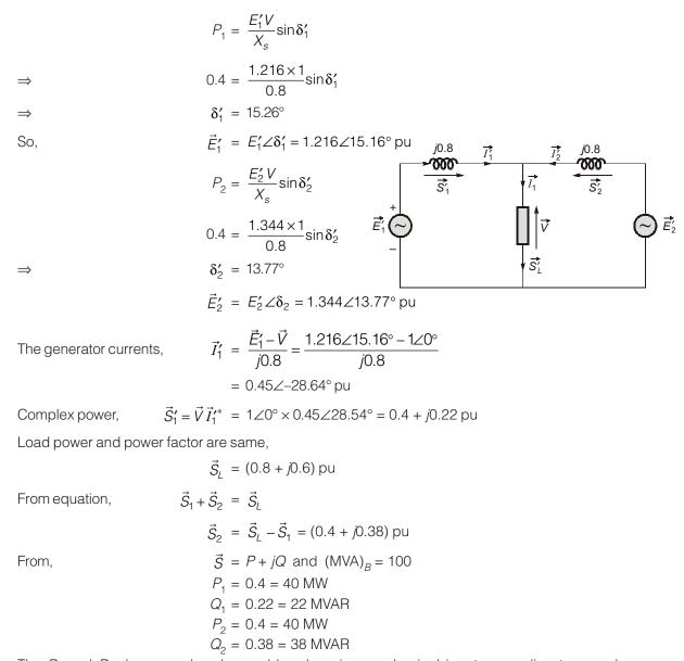
The  $P_1$  and  $P_2$  share can be changed by changing mechanical input, according to speed governer characteristics.
