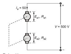
$$E_{a1} + E_{a2} + I_a(R_{a1} + R_{a2}) = V$$
