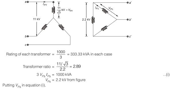
$I_{P\Delta} = \frac{1000}{3 \times 2.2} = 151.51 \text{ A}$  $I_{PY} = \frac{151.51}{2.88} = 52.60 \text{ A}$  $V_{PY} = \frac{11}{\sqrt{3}} = 6.35 \text{ kV}$
