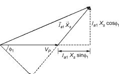
For synchronous reactance,  $X_{\rm S} = 0.25$  pu
