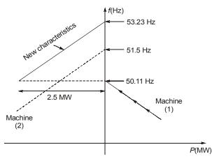
Whereas for generator '2' the total load = 2.5 MW operating at f = 50.11 Hz Now the no load frequency of generator '2';  $f_{0_2}$
