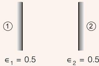
$$Q_1 = \frac{\sigma A(T_1^4 - T_2^4)}{\left(\frac{1}{\epsilon_1} + \frac{1}{\epsilon_2} - 1\right)} = \frac{\sigma A(T_1^4 - T_2^4)}{3}$$
