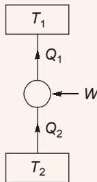
$$\text{COP} = \frac{T_1}{T_1 - T_2}$$
