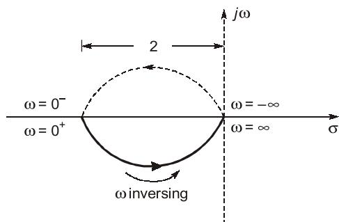
No roots of the characteristic equations are laying on the right hand side of the s-plane, therefore, closed-loop system is stable.
