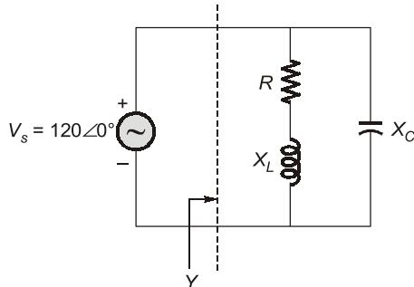
$Y$  = equivalent admittance of the parallel circuit
