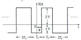
In this binary wave, logic-1 is represented with positive rectangular pulse and logic-0 is represented with negative rectangular pulse, both with different amplitudes.  $\phi$  is an independent random variable uniformly distributed in the range  $[0, T_b]$ , where  $T_b$  is the bit duration. Determine and sketch the auto-correlation function of X(t). Assume that logic-1 and logic-0 are occurring with equal probability.
