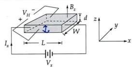
The device has dimensions  $d = 5 \times 10^{-3}$  cm,  $W = 5 \times 10^{-2}$  cm and L = 0.5 cm. The electrical parameters measured as the result of the experiment are  $I_x$  = 0.5 mA,  $V_x$  = 1.25 V and  $B_z = 6.5 \times 10^{-2}$  T. If the induced Hall electric field is  $E_{Hy} = -16.5$  mV/cm, then determine:
