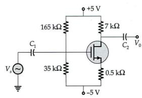
The transistor parameters are  $V_{TN}$  = 0.8 V,  $K_n = \frac{\mu_n C_{ox} W}{2L} = 1 \, \text{mA/V}^2$  and  $\lambda = 0$ .
