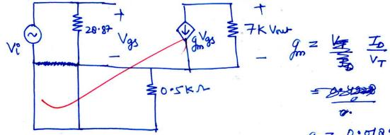
$$\frac{V_{out}}{V_i} = \frac{-g_m 7}{1 + g_m 0.5} = \frac{-7 g_m}{1 + g_m 0.5} = \frac{-0.1326 \times 1000}{10.457}$$
