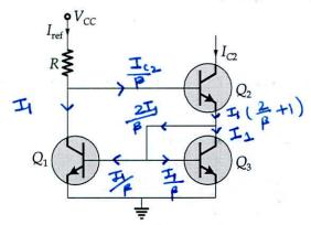
Assume that the three transistors to be matched with  $V_{BE1} = V_{BE3}$  and  $\beta_1 = \beta_2 = \beta_3 = \beta$ . Derive an expression for  $I_{C2}$  in terms of  $I_{ref}$ .
