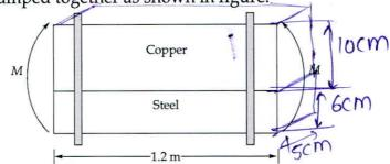
Both are of equal length and both have 5 cm width. Height of copper beam is 10 cm and that of steel beam is 6 cm. What could maximum moment that can be allowed without any failure of  $E_{\text{Cu}} = 120\,\text{GPa}$ ,  $(\sigma_{\text{allowable}})_{\text{Cu}} = 150\,\text{MPa}$ ,  $E_{\text{St}} = 200\,\text{GPa}$  and  $E_{\text{Cu}} = 120\,\text{GPa}$ .
