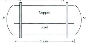
Both are of equal length and both have 5 cm width. Height of copper beam is 10 cm and that of steel beam is 6 cm. What could maximum moment that can be allowed without any failure of  $E_{\text{Cu}} = 120 \,\text{GPa}$ ,  $(\sigma_{\text{allowable}})_{\text{Cu}} = 150 \,\text{MPa}$ ,  $E_{\text{St}} = 200 \,\text{GPa}$  and  $(\sigma_{\text{allowable}})_{\text{St}} = 250 \,\text{MPa}$ ?
