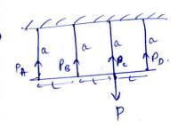
a- area j of wires. e- length E- pplymy Static Equalibrium EFy=0
