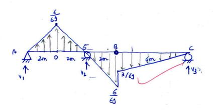
$$V_{1}+V_{2}+V_{3} + \frac{1}{2} \times 4 \times \frac{6}{63} = \frac{1}{2} \times 2 \times \frac{6}{63} + \frac{1}{2} \times 6 \times \frac{3}{63}$$
