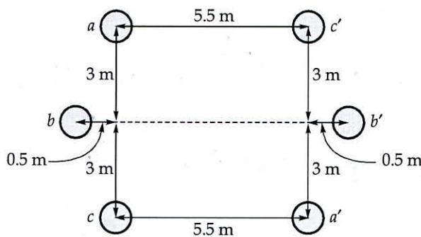
$$D_{ab} = \sqrt{3^2 + (0.5)^2} = 3.041 \text{ m}, \quad D_{ab'} = \sqrt{3^2 + 6^2} = 6.708 \text{ m} \quad [20 \text{ marks}]$$
