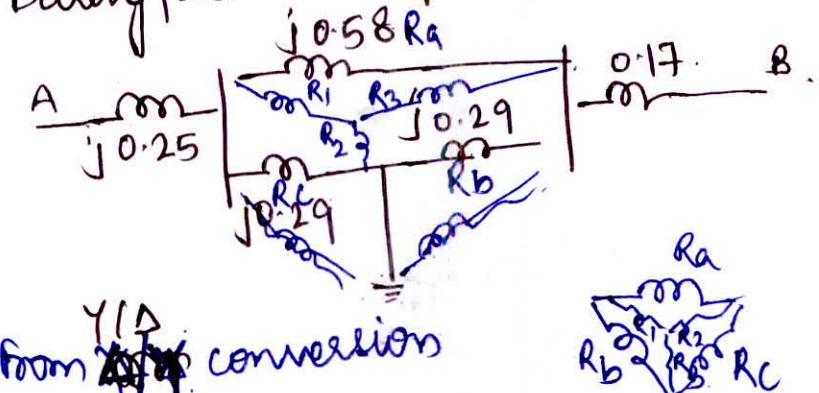
$$R_1 = R_a + R_b + \frac{R_a R_b}{R_c}$$
