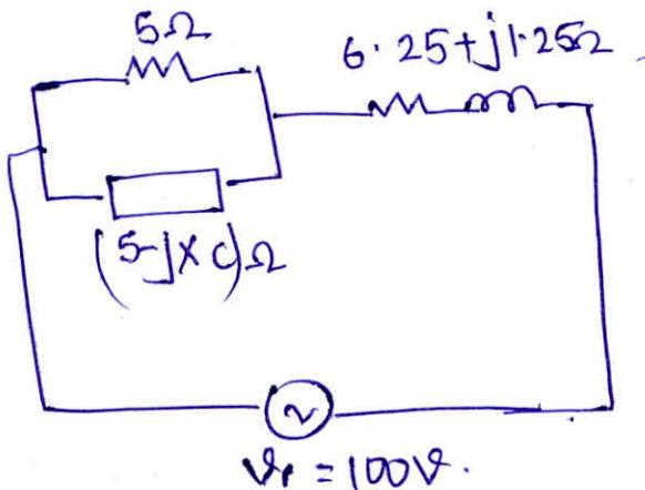
for resonance Imaginary part of equivalent input impedance should be zero.
