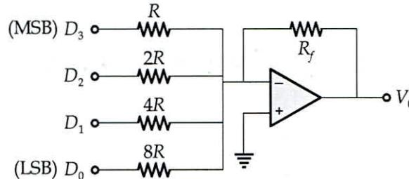
4 bit weighted resistor type DAC.
