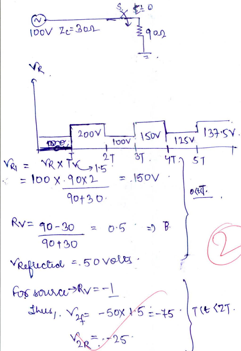
$$2T < t < 3T \quad V_{2f} = 25 \times 1.5 = 37.5$$
