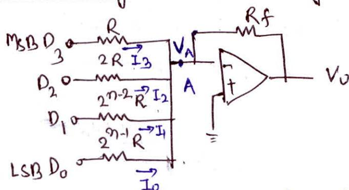
The  $D_3, D_2, D_1, D_0$  bits are either connected to  $V_{CC}$  or to ground. Let the voltage at A be  $V_A$ .
