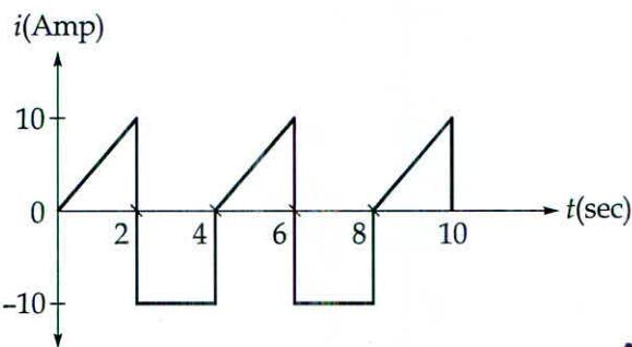
$$I_{rms} = \left[ \frac{1}{T} \left( \int_0^2 (5t)^2 dt + \int_2^4 (-10)^2 dt \right) \right]^{1/2} \quad [12 \text{ marks}]$$
