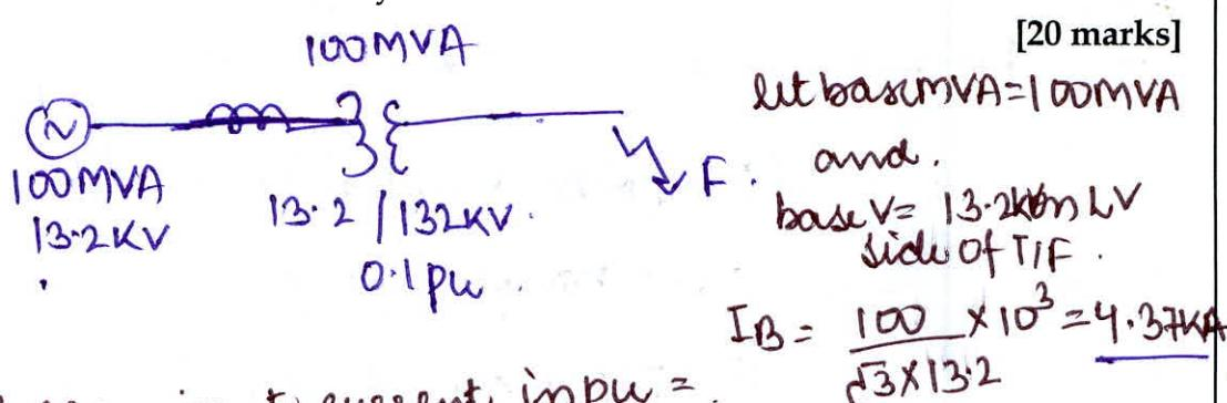
(i). Subtransient current in pu =
