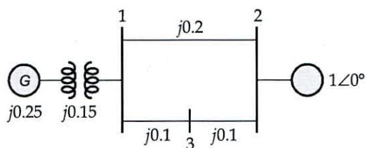
All the values are in per unit on a common base. The power delivered into bus-2 is 1.0 p.u. at 0.8 p.f. lagging. Obtain the power angle equation and swing equation of the system. Neglect all losses.
