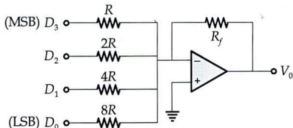
i) Four bit weighted resistor type DAC [12 marks]
