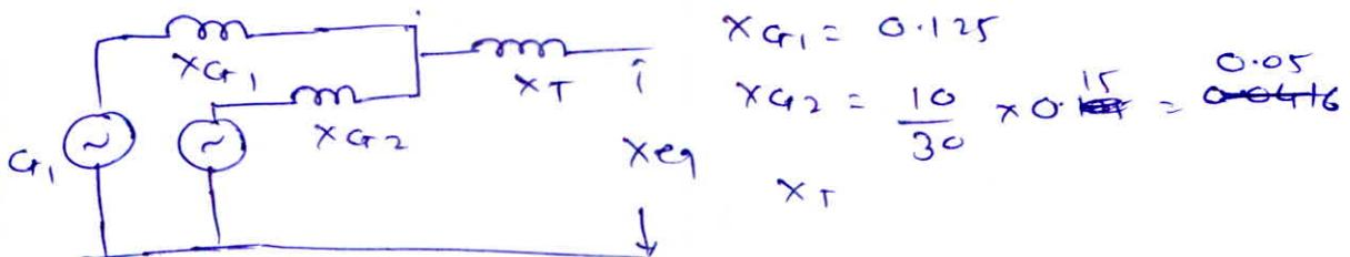
For fault on secondary bus of Transformer,
