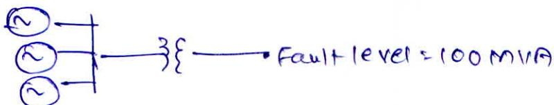
Reactance diagram :  $S_b = 30 \text{ MVA}$
