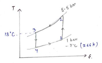
Assuming process 1-2 Mentropie;  $T_{p} = \begin{pmatrix} \rho_{2} \\ \overline{\rho}_{1} \end{pmatrix}^{\frac{y-1}{y}}$   $T_{p} = 266 \begin{pmatrix} 5.5 \end{pmatrix} \frac{1.4-1}{1.4}$
