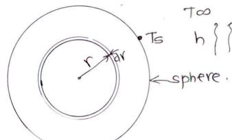
fora sphese the onedimensional Radi-al Heat conduction with uniformly Heat generation is given by
