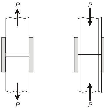
Generally the exact load carried by a splice is uncertain. Thus tension splice is designed for a design load or 0.3 times the member design capacity, whichever is more. It is always beneficial to design the splice for the strength of the member.
