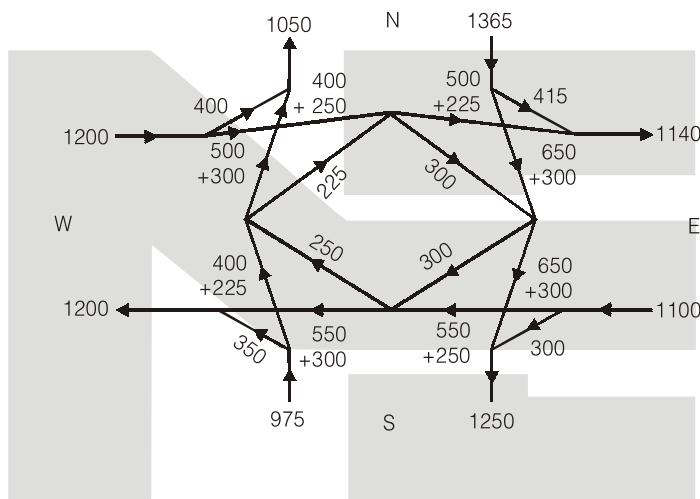
The maximum 2 way flow in the intersection leg (North) is 2415 PCU/hr and the maximum in one direction is 1365 PCU/hr.
