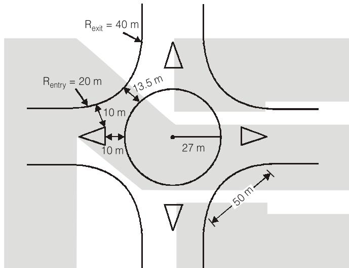
The radius of rotary at exit is taken as 2 times the radius at entry i.e.  $2 \times 20 = 40 \text{ m}$
