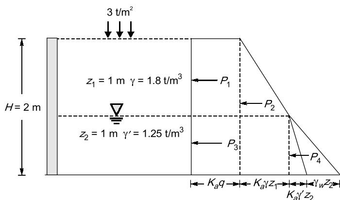
$$\text{Active Pressure, } P_1 = K_a q z_1 = \frac{1}{3} \times 3 \times 1 = 1 \text{ t/m at } \left(1 + \frac{1}{2}\right) m \text{ from base}$$
