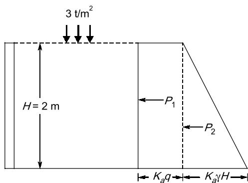
**Active thrust:**  $P_1 = K_a q H = \frac{1}{3} \times 3 \times 2 = 2 \text{ t/m}$  at  $\frac{H}{2}$  from base i.e. 1 m from base.
