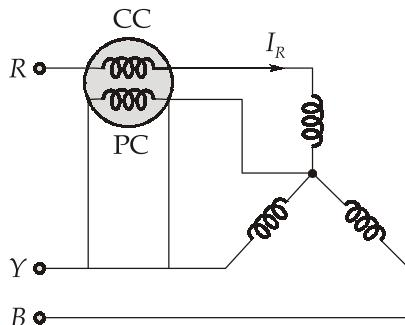
$$V_{YB} = V_Y - V_B = V\angle -120^\circ - V\angle -240^\circ$$
