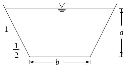
$$\text{Side slope of channel} = \frac{1}{2} H : 1V$$
