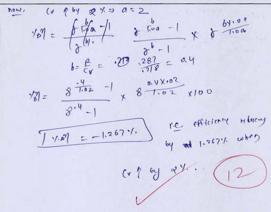
A passout two stage turbine receives steam at 50 bar and 350°C. At 2.0 bar the high-pressure stage exhausts and 12000 kg of steam per hour are taken at this stage for process heating. The remainder is reheated at 2.0 bar to 250°C and then expanded through the low pressure turbine to condenser pressure of 0.05 bar. The power output from the turbine unit is 3750 kW. Take isentropic efficiency of high pressure and low pressure turbine stage as 0.81. Calculate the boiler capacity.
