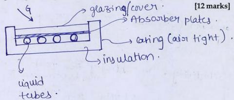
when solar inso vatton strikes the liquid when solar inso vatton strikes the liquid fat plate collector, some part of it gets absorbed in the absorber plate. This heat absorbed in the absorber plate. This heat is then transferred to heat transfer founds is then transferred to heat transfer founds which can then be used too required which can then be used too required application.
