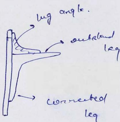
\* The outstand leg of the member does not impact in carrying load upto its full capacity.
