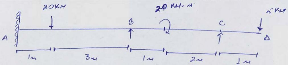
$$M_{FAB} = -\frac{20 \times 1 \times 3 \times 3}{4 \times 4} \Rightarrow -11.25 \text{ KN-m}$$
