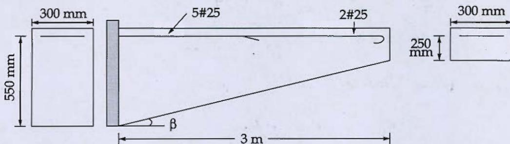
Design shear strength for M25 grade concrete.
