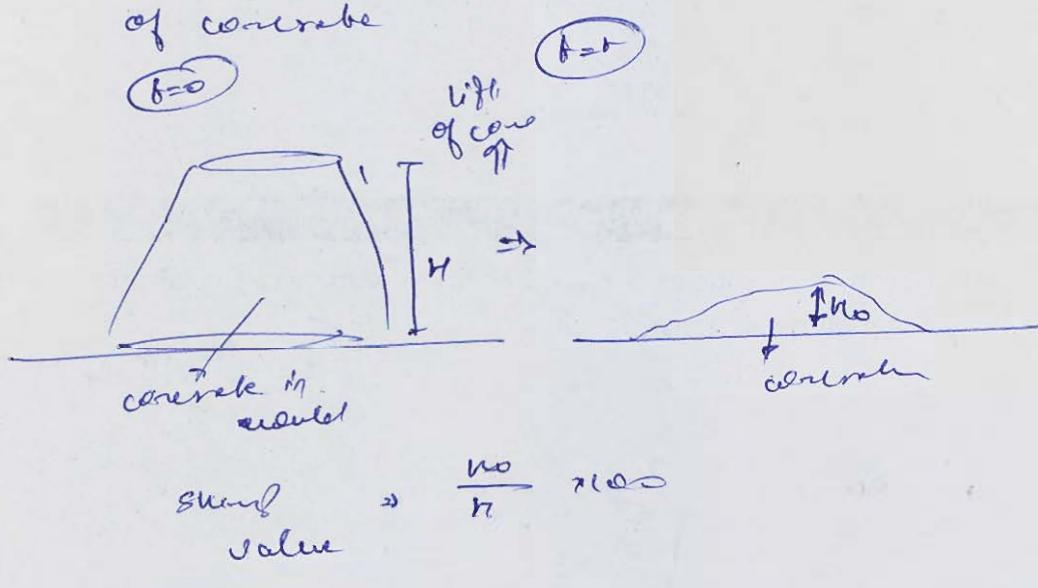
$\Rightarrow$  calibration is done to find the workable height with the shrinkage value.
