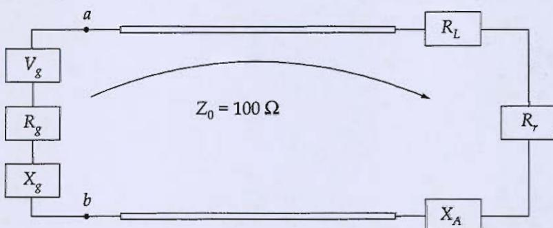
Determine the power radiated by the antenna (Given,  $V_g = 10 \text{ V}$ ,  $R_g = 50 \Omega$ ,  $X_g = 0$ ).
