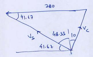
$$\frac{V_{c}}{Sin(41.67)} = \frac{280}{Sin(48.33+10)} = \frac{V_{S}}{Sin(80)}$$
