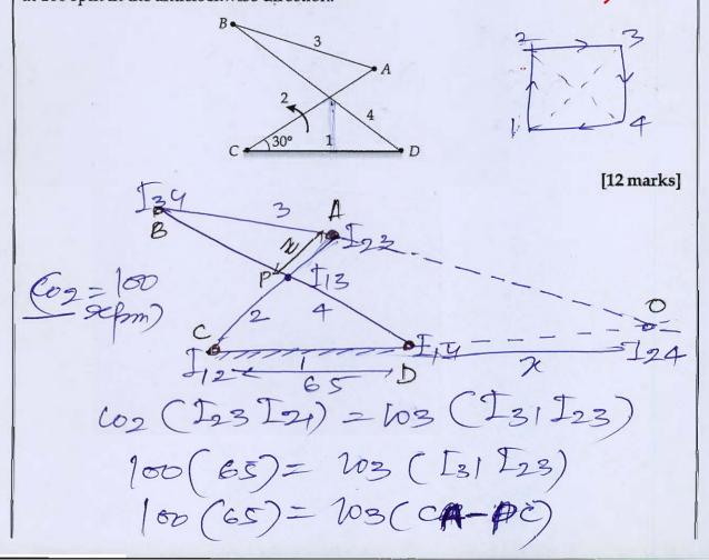
From Leage (PCD) CBC0830 = CP CBX 13/5 = CP CP = 53.65 100×65=103(60-13×65) la x65= Wz (60-56-29) N3=17-52-02 95m (03=183-47-900) APZZ=(60X)-13x65) =3.908 from Figure APB and BDO BP = BD 204 = 20DB PA DO  $lo_2(I_{24}I_{21}) = lo_4(I_{24}I_{41})$   $2\pi \times loob)(65+2) = loo4(2)$ BP = 80 3.708 2
