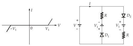
**2.** To achieve the given characteristics, we need two diodes  $D_1$  and  $D_2$  connected in parallel. The diode  $D_1$  is forward biased when V > 0 and diode  $D_2$  is forward biased when V < 0. Since the current is non-zero for V = 0. Thus, we place the current sources as shown in the figure below.
