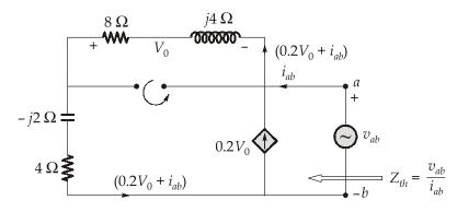
Applying KVL around the loop,
