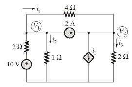
Apply KCL at node  $V_1$ :
