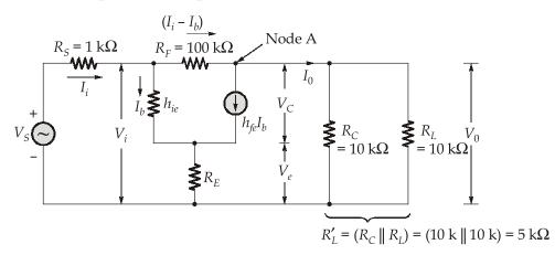
Step 2: Apply KVL to the output loop,
