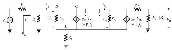
(ii) Input resistance  $R_{\text{in}} = \left(\frac{V_{in}}{I_{b_1}}\right) || (R_1 || R_2)$
