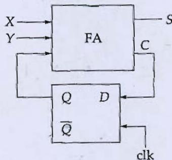
5) (e) Given: circuit with full adder and D flip flop.
