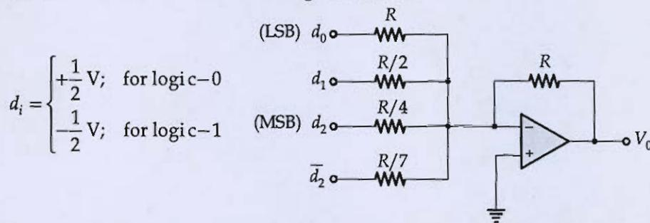
Derive an expression for output voltage  $V_0$  in terms of input logic values. Using the result obtained, determine the value of  $V_0$  for all the possible binary combinations of input and comment on the operation performed by the circuit.
