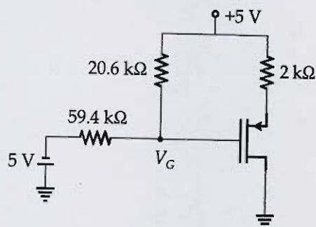
The transistor parameters are  $V_{TP} = -1.5$  V and  $\frac{\mu_p C_{ox} W}{2L} = 0.5$  mA/V<sup>2</sup>. Calculate:
