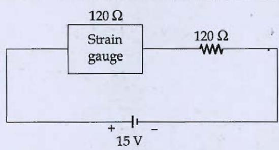
Calculate the difference between the output voltage (voltage across the strain gauge) with no stress applied and with a stress of  $150 \text{ MN/m}^2$ . The modulus of elasticity of the material undergoing strain is  $200 \text{ GN/m}^2$ .
