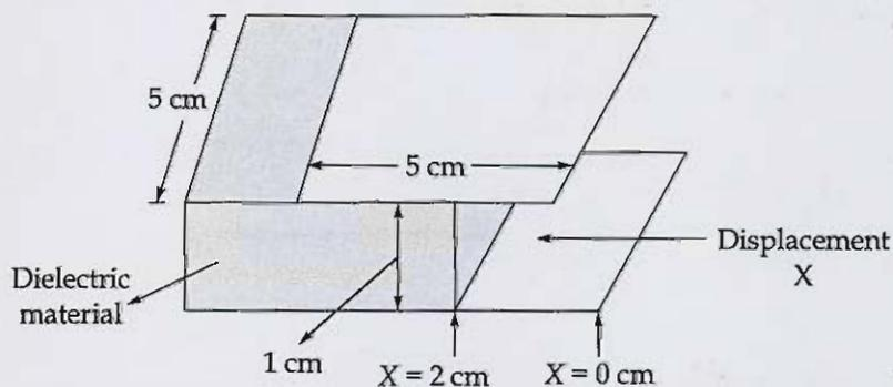
The parallel plate has a dimension of 5.0 cm  $\times$  5.0 cm and is separated by a distance of 1.0 cm. The space between the plates is filled with a dielectric material 1.0 cm thick, which has a dielectric constant of 4.0. If dielectric constant for air is 1.0, determine the value of the capacitance when  $X$  is equal to
