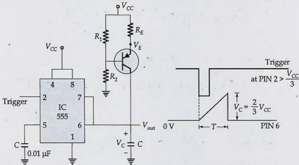
Determine the time period ( $T$ ) of ramp waveform.
