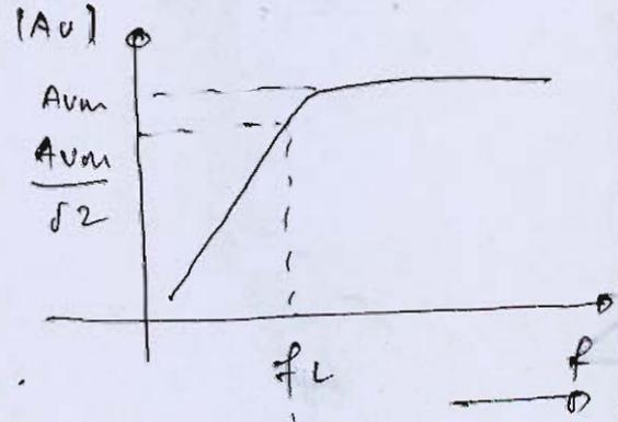
$$A_v(s) = \frac{-\beta R_e R_B}{r_n + (1+\beta)R_e} \left( \frac{1 + (R_B + R_S)C_S}{C_S} \right)$$
