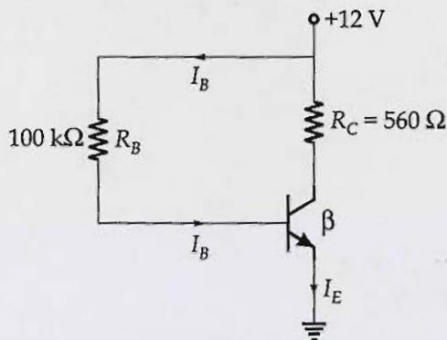
(Neglect any change in  $V_{BE}$  and the effects of any leakage current)
