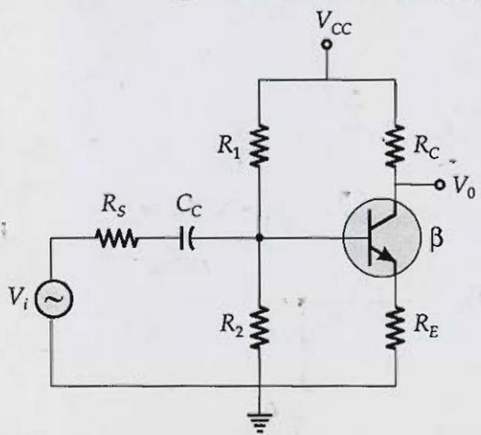
Derive the expression for the overall voltage gain of the transistor  $A_V(s)$  as a function of input capacitance  $C_C$ . Also draw the approximate magnitude plot for the voltage gain  $A_V(s)$ . [Assume  $V_A = \infty$ ]
