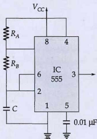
where,  $R_A = 2.2 \text{ k}\Omega$ ,  $R_B = 3.9 \text{ k}\Omega$  and  $C = 0.1 \mu\text{F}$
