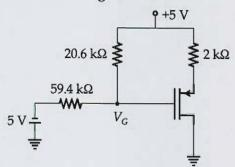
The transistor parameters are  $V_{TP} = -1.5 \text{ V}$  and  $\frac{\mu_p C_{ox} W}{2L} = 0.5 \text{ mA/V}^2$ . Calculate:
