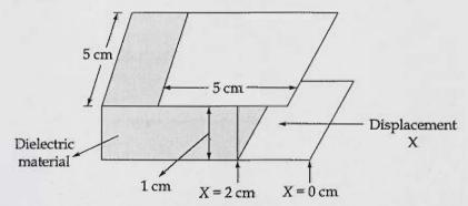
The parallel plate has a dimension of 5.0 cm × 5.0 cm and is separated by a distance of 1.0 cm. The space between the plates is filled with a dielectric material 1.0 cm thick, which has a dielectric constant of 4.0. If dielectric constant for air is 1.0, determine the value of the capacitance when X is equal to
