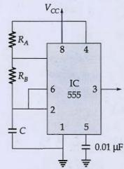
where,  $R_A$  = 2.2 k $\Omega$ ,  $R_B$  = 3.9 k $\Omega$  and C = 0.1  $\mu F$
