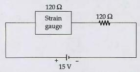
Calculate the difference between the output voltage (voltage across the strain gauge) with no stress applied and with a stress of  $150\,\mathrm{MN/m^2}$ . The modulus of elasticity of the material undergoing strain is  $200\,\mathrm{GN/m^2}$ .
