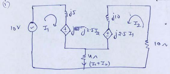
$$\frac{9n \text{ Joop } -1}{-10 + j5 \text{ J}_1 + j2.5 \text{ J}_2 + 4(\text{J}_1 + \text{J}_2) = 0}$$
