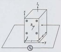
State what happens when magnetic field  $B_z$  is applied in positive z-direction in reference to Hall voltage. Determine electron mobility relation using Hall coefficient and conductivity ( $\sigma$ ).
