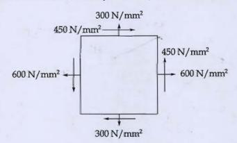
Determine the normal and tangential stresses on the two planes which are equally inclined to the planes carrying normal stresses mentioned above.
