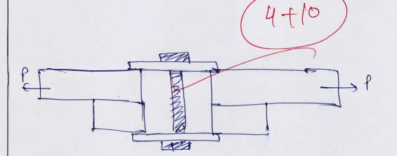
load transfer is through fretional force generated in balt.
