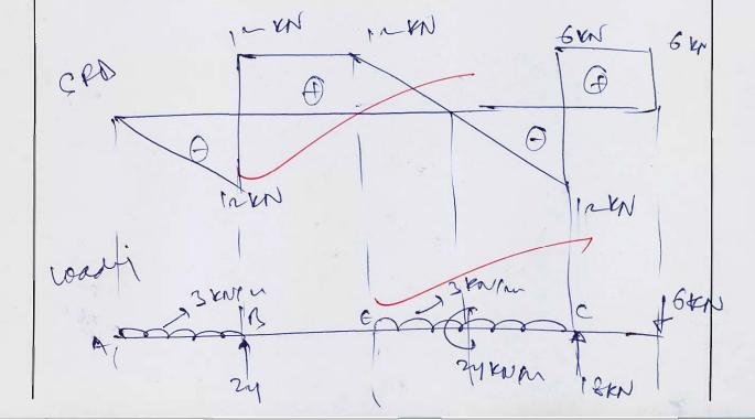
Q.8 (b) For the beam as shown in figure, compute the ordinate of influence line for  $R_A$  at 1 m interval. Assume EI of beam is constant.
