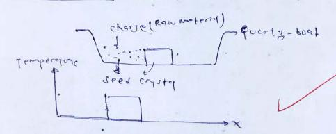
charge is keept into molter state.
