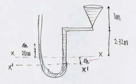
Equating pressure at x'-x' from both sides
