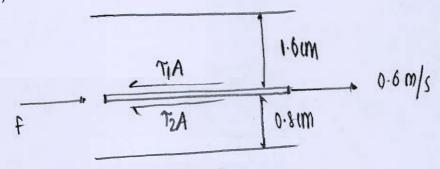
$$T_1 = \frac{\mu dv}{dV_1} = \frac{0.81 \times 0.6}{1.6 \times 10^{-2}} = \frac{30.375 \, \text{N/mm}^2}{1.6 \times 10^{-2}}$$
