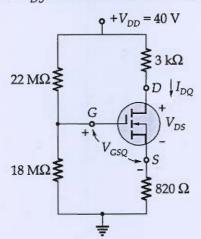
$V_{GS \text{ (Th)}} = 5 \text{ V}, I_D(\text{on}) = 3 \text{ mA at } V_{GS}(\text{on}) = 10 \text{ V}.$
