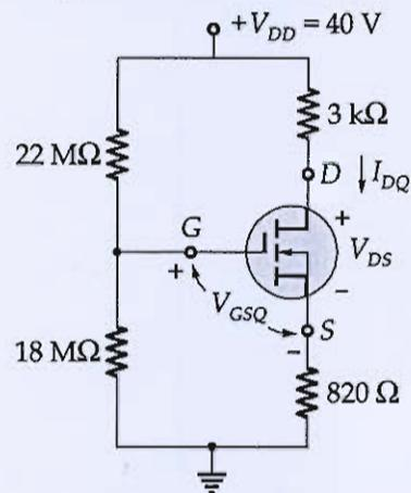
$V_{GS(Th)} = 5 \text{ V}$ ,  $I_{D(on)} = 3 \text{ mA}$  at  $V_{GS(on)} = 10 \text{ V}$ .
