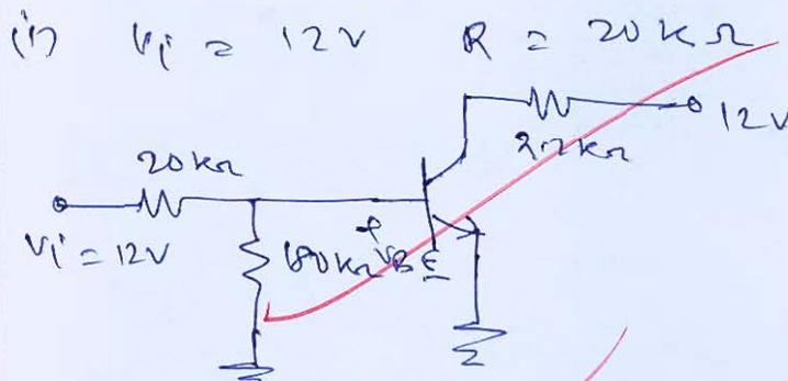
$$V_{th} = 12 \times \left( \frac{180}{180 + 20} \right) = 10.8 \text{ V}$$
