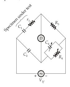
$$r_1 = \frac{C_4}{C_2} R_3 = \frac{0.5 \times 10^{-6}}{106 \times 10^{-12}} 260$$
