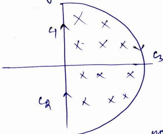
\* Since the given system contains 1 pole (open loop) in the right side of the s-plane,
