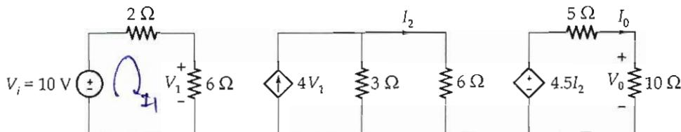
Determine the output voltage ( $V_0$ ), output current ( $I_0$ ) and voltage gain ( $V_0/V_i$ ).
