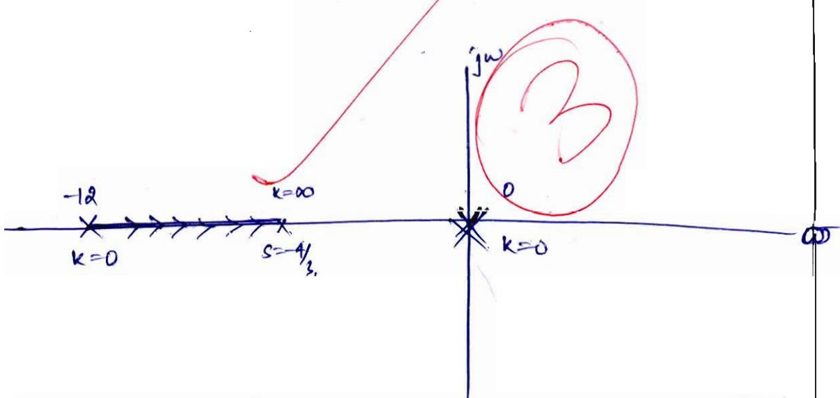
\* Root locus exists only for those portions on the real axis where the no. of poles and zeros are odd to the right of the point.
