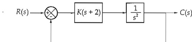
Determine the value of  $K$  such that the phase margin of the system is  $50^\circ$ .
