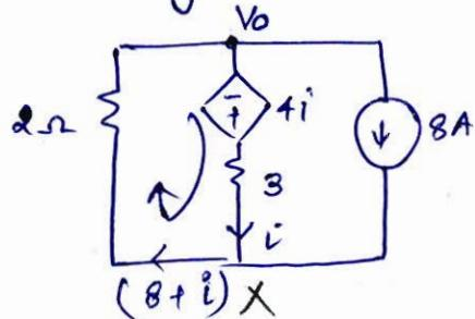
applying the KCL at node  $V_0$ ,
