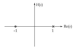
Since the system is given to be stable, the ROC of the impulse response must include the  $j\omega$  axis. Thus, the ROC of H(s) has to be Re $\{s\}$  < 1.
