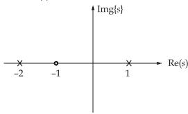
Since the given system is a causal system, the ROC of the impulse response is right-sided. Thus, from the given H(s), the ROC is  $Re\{s\} > -1$ . We know that the ROC of Y(s) is at least the intersection of the ROCs of X(s) and Y(s).
