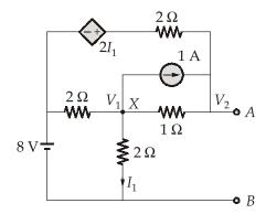
Let the voltage at node X be  $V_1$  and that at terminal A be  $V_2$ .
