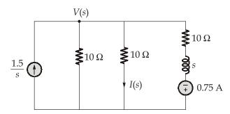
$\therefore$  Applying KCL analysis at node V(s),
