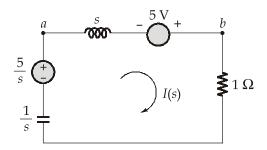
Transforming the voltage sources into current sources we have the network
