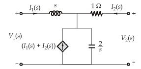
By using source transformation theorem, we can redraw the given two port network as
