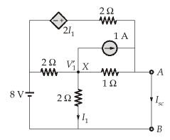
Let the voltage at node X be  $V'_1$ . Using nodal analysis at node X, we obtain
